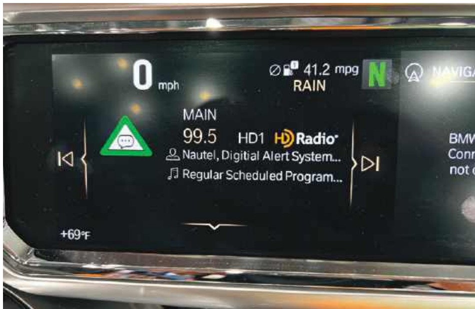
Below and Right Fig. 9: Consumer HD Radio receivers showing alert graphics and text.
