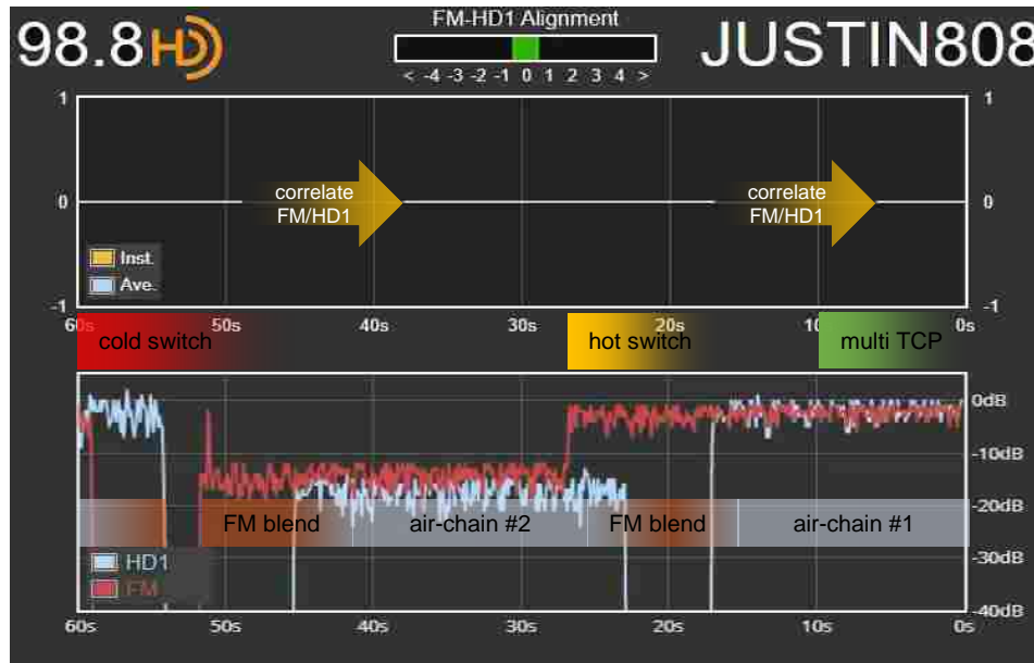
FIGURE 9: CONSISTENT FM-HD1 ALIGNMENT ACROSS CHANGEOVER. A COLD STANDBY CHANGEOVER MAY CAUSE SHORT SILENCE WITHOUT RF CARRIER DROP, A HOT STANDBY CHANGEOVER BLENDS GRACEFULLY TO THE FM CONTENT, A MULTIPLE TCP CHANGEOVER TO THE SAME AIR-CHAIN IS HITLESS.
