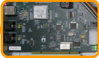
Integrated GPS receiver 1 PPS is system heart beat Ovenized 10 MHz Crystal
