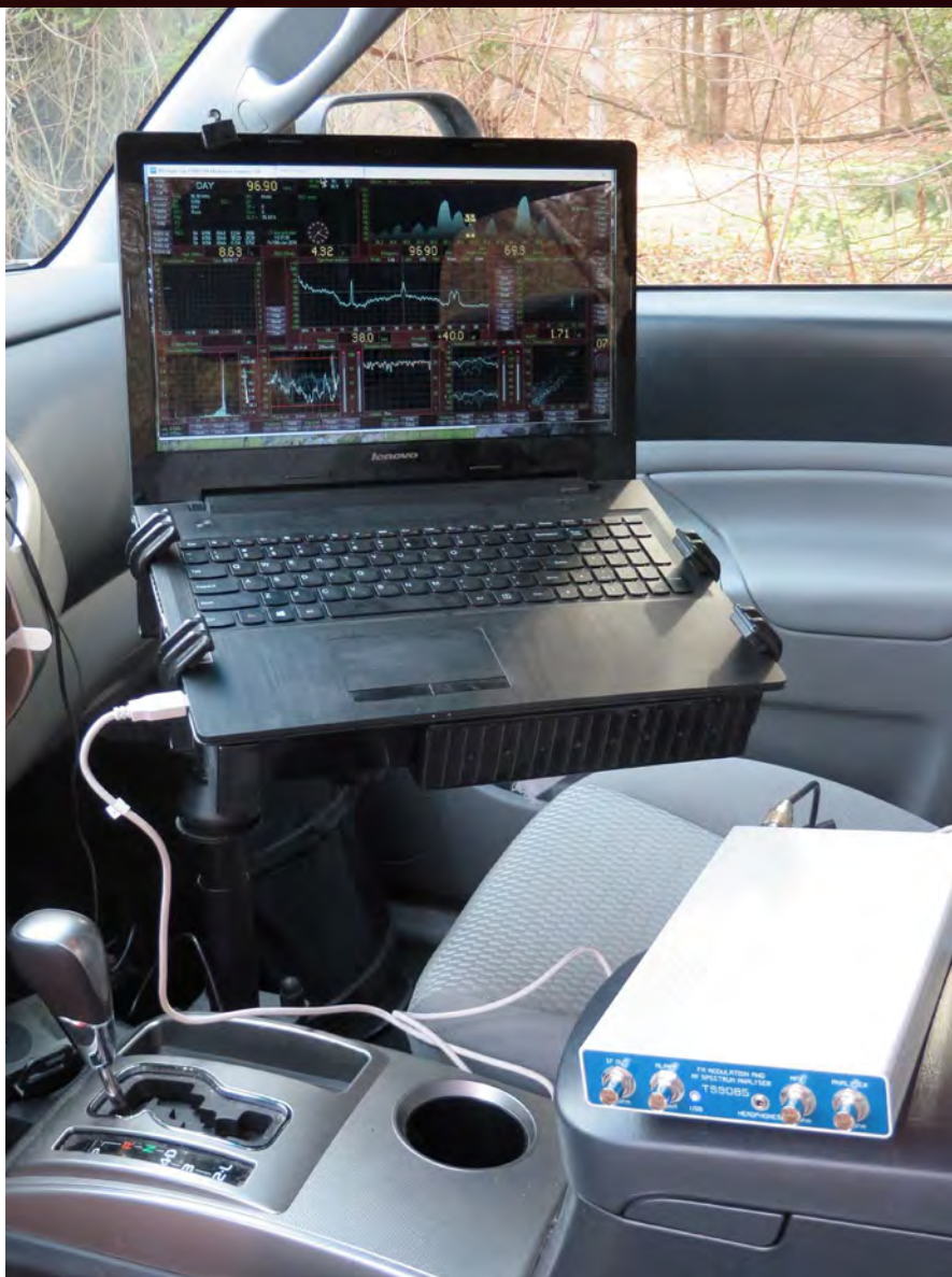
Fig. 1: Tools of the trade — typical equipment setup for mobile FM field strength measurements in the cab of a truck.
