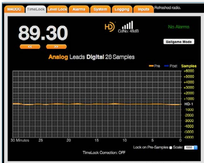
HD Radio time alignment is demonstrated here using DaySequerra diversity delay control at KUVU(FM) in Denver.
