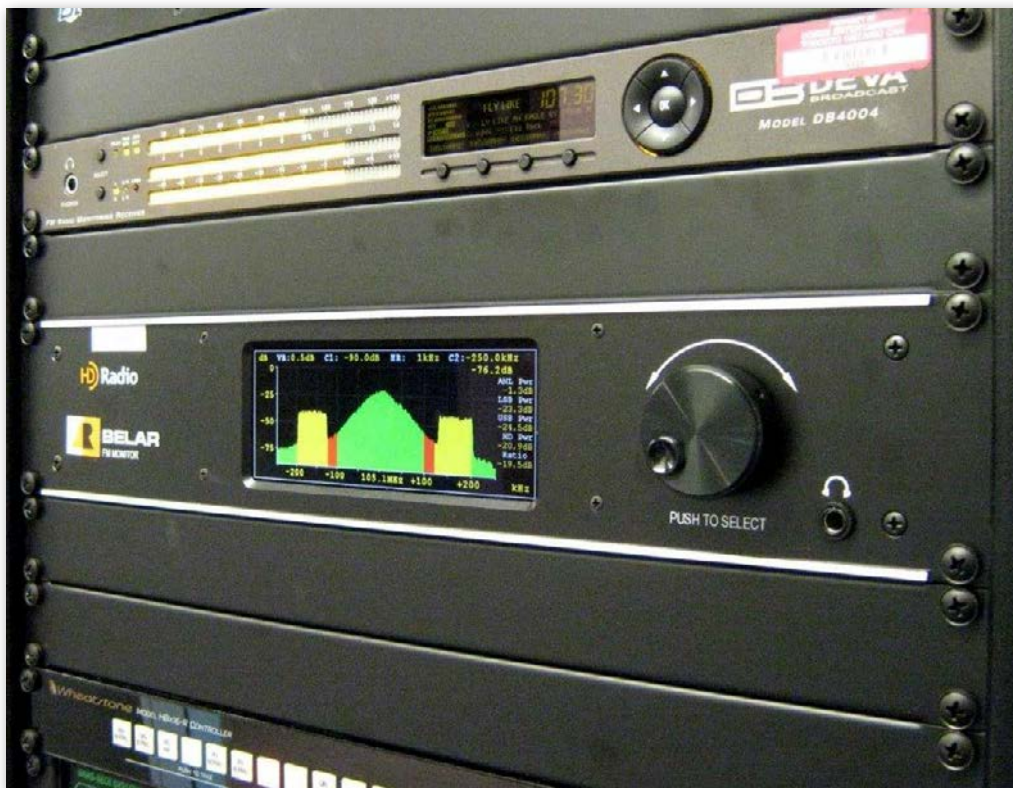
Modulation monitor shows an HD signal for a Corus station.
